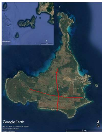
Fig. 1: The island of Pianosa and its position in the Tuscan Archipelago. (Google Earth, 2024). Red lines are the ERT surveys acquired in 2023 (NS oriented) and in 2024. The point shows the location of the borehole ERT.
